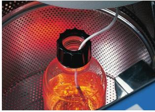
**Pt 100 Sensor.** 2<sup>nd</sup> Probe for reading sample temperature.
